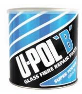
U-POL polyester glass fibre filler is a two component chemical paste with glassfibre strands (chop strand mat) used for bridging of holes and rust in surfaces such as steel and GRP. U-POL forms a very hard, durable surface and can be sanded and shaped if required. It is easily covered with standard polyester filler or can be over-painted with most common paints.
