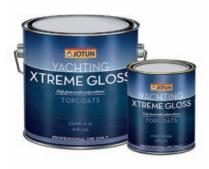
This is a two component chemically curing acrylic polyurethane coating. It is an abrasion resistant high solids product. It has a high gloss finish with excellent gloss retention. To be used as topcoat in atmospheric environments. For exterior areas, including hull, above waterline and superstructure. The Jotun Xtreme Gloss paints can be tinted to many BS, RAL and Jotun colours.
