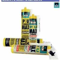
One-component thixotropic polyurethane adhesive, setting when exposed to atmospheric moisture or by material humidity. Will bond wood, concrete, expanded polyurethane, formica and metals on porous substrates.
