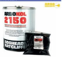
Arbokol 2150 is a two component, hard wearing structural polysulphide adhesive. Arbokol 2150 is ideal for hull-to-keel joints and swimming pool joints. Arbokol 2150 is not recommended for large joints with large amounts of movement.
