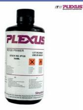
Primer/Conditioner for non-porous metals to allow better bond strength for Plexus products outside the 800 series. Wipe on and leave for 120 seconds to flash off.
