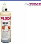
A high strength 10:1 structural adhesive. Plexus MA320 has excellent low temperature properties. Working Time - 8-12 minutes. Fixture Time - 25-30 minutes. Gap Fill - 10mm.
