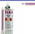
Medium open time, high strength 10:1 metal bonder. Can be used without the need prime. Working Time - 12-16 minutes. Fixture Time - 50-60 minutes. Gap Fill - 12 mm
