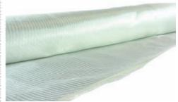
These non-crimp fabrics combine two layers of unidirectional fibres 45° which are stitched together using a light thread. The result is an engineered biaxial fabric with predictable, repeatable properties.
