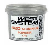
Add between 5% to 10% by volume to provide protection from ultraviolet light in areas which will not be protected with other coatings or as a base for subsequent painting. Will substantially increase the hardness of the coated surfaces.
