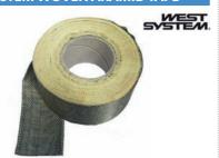
Aramid fabric provides excellent abrasive and tear resistance in addition to good impact resistance due to its ability to absorb and dissipate energy. Woven aramid tape is excellent for providing extra strength in localised high wear areas such as canoe and kayak keel lines, etc. 0.39mm thickness. Available in 50mm and 75mm widths.
