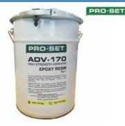
This pre-thickened, 1:1 mix, two part epoxy system is Lloyds Register of Shipping approved for the bonding of teak planking to glass reinforced polyester decks. Both resin & hardener are thixotropic pastes, resulting in good gap fill and sag resistant properties. Pro-Set 170/270 will also bond a wide variety of other substrates such as concrete, metals, and composites.
