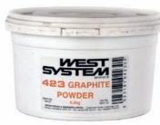
A fine black powder added to West System epoxy to produce a low-friction exterior coating with increased scuff resistance, durability and mar-resistance. Graphite Powder is often used for coating the bottom of rudders and centre boards or the bottom of racing crafts which are dry sailed from the beach. Graphite Powder can also be used in teak deck construction to simulate traditional seams in appearance. Add 10% by volume to mixed epoxy.
