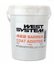
A proprietary blend designed to improve the moisture-exclusion effectiveness of West System epoxy and to combat osmosis. It is an excellent additive for providing a barrier coating to overcome gelcoat blistering and also increases the abrasion resistance. Add 20% to 25% by weight to the mixed epoxy.
