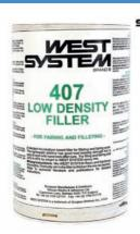
A blended microballoon-based filler to make fairing putties which are easy to sand but remain strong on a strength-to-weight basis. Add 20% to 40% by weight to mixed epoxy. Colour: Reddish-Brown.
