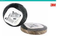
Safety-Walk General Purpose Slip Resistant Surfacing is a high-friction textured material. It consists of abrasive mineral particles bonded by a tough, durable polymer to a dimensionally stable plastic film. The backing is coated with a pressure-sensitive adhesive covered by a removable protective liner.
