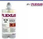
An all purpose, high strength 1:1 structural adhesive. Plexus MA300 will bond a range of plastics and metals (with the use of the metal primer PC120). Working Time - 4-6 minutes. Fixture Time - 12-15 minutes. Gap Fill - 4mm.
