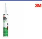
A one part general purpose polyurethane that chemically reacts with moisture to deliver flexible bonds with good adhesion to wood, fibreglass, gelcoat, certain plastics and metals.
