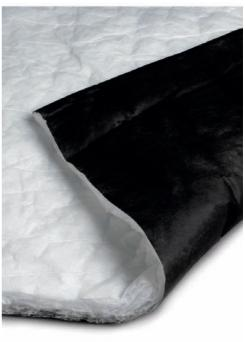
This non-woven matt has excellent sound absorbing properties useful in many interior applications, for example inside door panels, instrument panels, pillar stuffers, and package trays. It is compressible, nonlinting, lightweight, and can be easily cut with scissors and/ or a knife. A black
