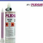
Medium open time, high strength 10:1 metal bonder. Can be used without the need prime. Working Time - 12-16 minutes. Fixture Time - 50-60 minutes. Gap Fill - 12 mm
