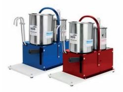
The West System 305 High-Capacity Positive Displacement Metering Pump dispenses five parts resin to one part hardener by volume. It consists of two separate parallel pump systems, one for the resin and one for the hardener. The two systems are operated simultaneously by a single lever. Blue Base. For use with 205 Fast or 206 Slow (5:1 ratio) Hardeners.
