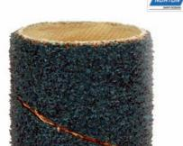
Spirobands are used for shaping holes cut into GRP to the correct shape using a drill or other power tool. The abrasive used is Zirconia meaning the cut lasts for a long time. Spirobands slip over and grip onto the Mandrill.
