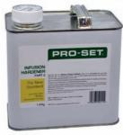
PRO-SET Infusion hardeners range from fast to extra slow, and may be blended to provide even greater versatility with your custom processes. PRO-SET 211 is the medium Infusion hardener with a working time of 3-4 hours at 25°C.
