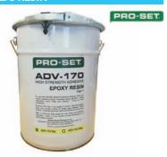
This pre-thickened, 1:1 mix, two part epoxy system is Lloyd's Register of Shipping approved for the bonding of teak planking to glass reinforced polyester decks. Both resin & hardener are thixotropic pastes, resulting in good gap fill and sag resistant properties. Pro-Set 170/270 will also bond a wide variety of other substrates such as concrete, metals, and composites.
