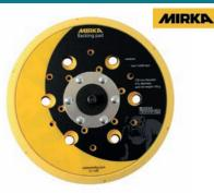
A 150mm backing pad with a central air inlet. The air channels leading to the centre of the backing pad has an increased air flow and therefore the dust is removed efficiently.
