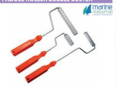
GRP Bubble Buster Rollers are manufactured from aluminium extrusion and have a secure screw fixing. It combines the advantages of the paddle roller with those of the finned roller. The same profile as the paddle roller but with a V-notch which reduces the amount of spray thus providing a consistent finish without air bubbles and allows flexible movement of fibre. Available with a long reach wire for hard to reach areas. Resistant to almost all cleaning agents.
