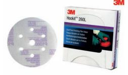
These discs are constructed of a high performance, aluminium oxide mineral bonded to a smooth film backing. Cuts fast, lasts long, resists loading and leaves a consistent finish. Primarily used for scuff sanding before painting, as well as to remove runs, dust, nibs and excess orange peel from paint and gelcoat prior to compounding. To be used with the 3M Soft Interface Pad (3M-50396).
