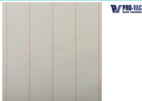
Peel Ply is a finely woven nylon or polyester fabric with an added release agent to which epoxy cannot bond. Apply Peel Ply to the surface of the wet epoxy and allow to cure. After the epoxy has set simply peel off the Peel Ply, which in turn will remove any surface Amine Blush, and you will be left with a woven impression resulting in no-need for washing and abrading between coats.
