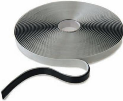
These specially designed putty tapes are ideal for creating an air-tight seal when vacuum bagging. They are pressure sensitive meaning that the harder you nip the tape to the bag, the better the seal you create. PRO-VAC 1191 General purpose Black low temperature sealant tape. Maximum use temperature 150°C.
