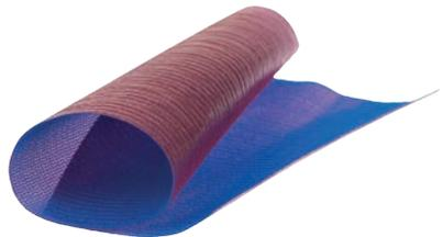
PRO-VAC RE-MESH - Release film and infusion mesh combination product. Combination of PRO-VAC 500-B-28-P31 release film and KM160E1 infusion mesh. Designed for resin infusion with a wide range of commonly used resin system. Reduces layup time and handling.
