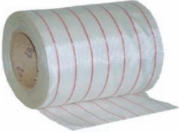
Peel Ply is a finely woven nylon fabric with an added release agent to which epoxy cannot bond. Apply Peel Ply to the surface of the wet epoxy and allow to cure. After the epoxy has set simply peel off the Peel Ply, which in turn will remove any surface Amine Blush, and you will be left with a woven impression resulting in no-need for washing and abrading between coats.
