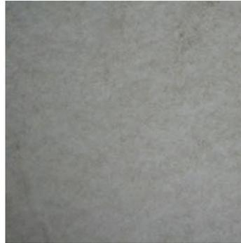
PRO-VAC Breather fabric is designed to aid in the evacuation of air from the dry composite fibres or pre preg layers during the de bulking process at room temperature; it also behaves as an open channel for gasses to escape during curing at elevated temperature and pressure whilst the laminate is still in its liquid phase before curing. PRO-VAC 150gsm non-woven polyester breather fabric. Maximum use temperature of 210°C. 100% non-woven polyester.
