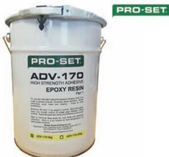
This pre-thickened, 1:1 mix, two part epoxy system is Lloyd's Register of Shipping approved for the bonding of teak planking to glass reinforced polyester decks. Both resin & hardener are thixotropic pastes, resulting in good gap fill and sag resistant properties. Pro-Set 170/270 will also bond a wide variety of other substrates such as concrete, metals, and composites.
