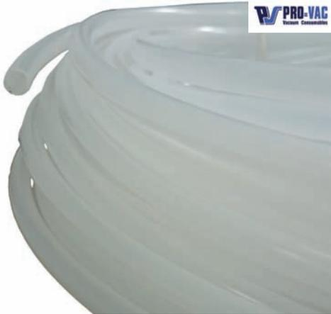
A plastic hose 12mm OD and 10mm ID designed to be used with resin infusion. Can be easily cut and kinked for stopping resin flow.
