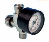
The Devilbiss air pressure gauge and regulator fits neatly inline at the gun air inlet, it increases or decreases the working pressure at the gun. Its calibrated up to 11 Bar (160 psi).
