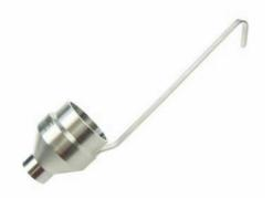
The TQC Viscosity Cup DIN 53211 Immersion is a titanium anodized aluminium viscosity cup with fixed stainless steel 4mm nozzle and handle. Ideal for measuring coatings and other fluids during application or production.
